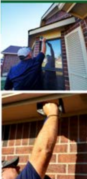
Certified Lead-Based Paint Inspector, Cody Regnier, operating a Heuresis Pb200i Handheld Paint Analyzer.
